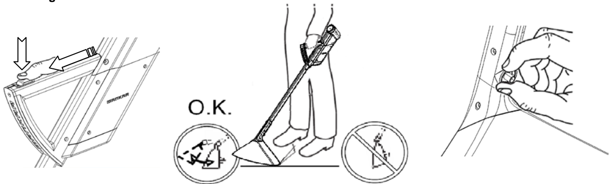
G: Setting of spray hood adjustment
